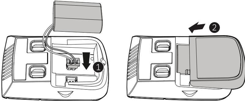
**Step 1:** Plug the battery connector securely into the socket inside the battery compartment. Insert the battery with the label **THIS SIDE UP** facing up onto the battery compartment.
